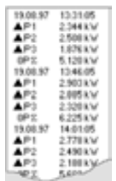
Measurement data can be recorded to the plug-in memory card or to recording chart paper at the integrated printer module.
